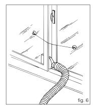
Pinguino is equipped with an adjustable window bracket. If you have a sash window, place the bracket on the window sill, extend the bracket fully within the window frame and lower the window onto the bracket. Insert the nozzle of the exhaust hose into the slot, then connect the hose to the air conditioner (Fig. 7).
